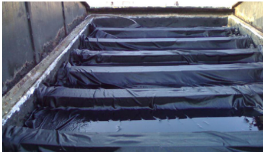
Figure 1.11: Solar still basin covered with a black cloth (figure by Murugavel and Sritharb [27]).
