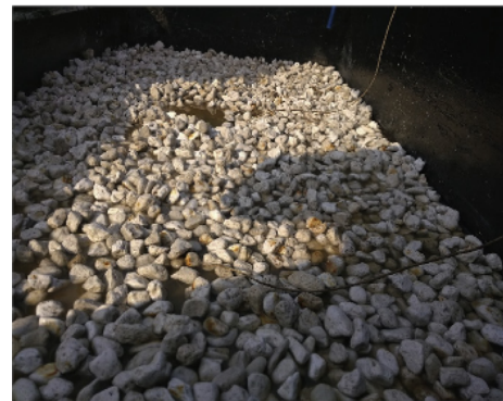
Figure 1.12: Solar still basin covered with pumice stones (figure by Bilal and Jamil [29]).
