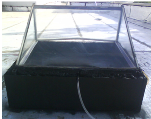
Figure 1.10: Single slope solar still with overall structure made of glass, and a sandy reservoir under the basin (figure by Tabrizi and Sharak [24]).
